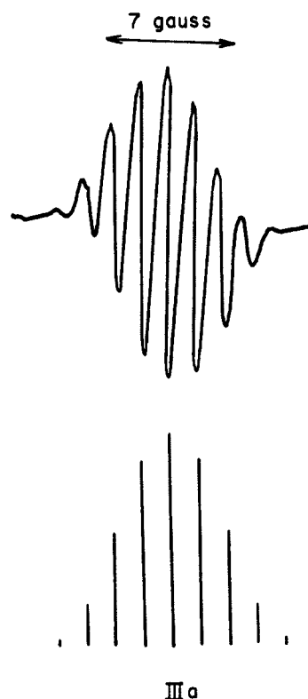
Figure 3.—First-derivative esr spectrum in benzene of libocedroxy radical (IIIa). The reconstructed spectrum is under the experimental spectrum. The center of lines is at approximately g = 2 .
